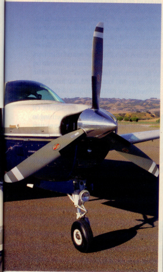
The IO-550 engine now has Superior Air Parts Millennium cylinders and is turbo-normalized with GAMInjectors installed (left). A Hartzell scimitar prop was also installed (above).
